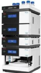
영문 장비명 : High-Performance Liquid Chromatography-UV-VIS Detectors (HPLC-UV-RI)
