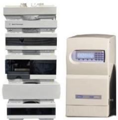
영문 장비명 : High-Performance Liquid Chromatography-Evaporative Light Scattering Detector (HPLC-ELSD)
